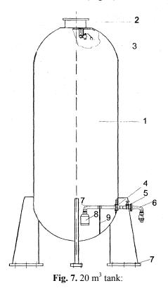
$1-20 \text{ m}^3$ tank; 2-drain cover; 3- overflow float value; 4- crossing piece;
